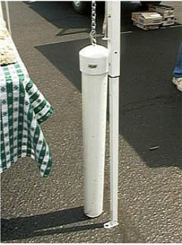
The PVC pipe filled with cement hangs on the inside of the canopy pole, and it has soft edges and the ability to move, just in case someone still manages to collide with it.
